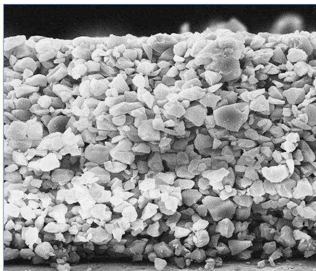
Electron microscope photograph of a cross section through an aluminium sheet with silica layer (magnification x 500)
