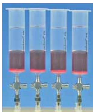
CHROMABOND® PTL in action: organic upper phase (colorless), aqueous lower phase (red)
